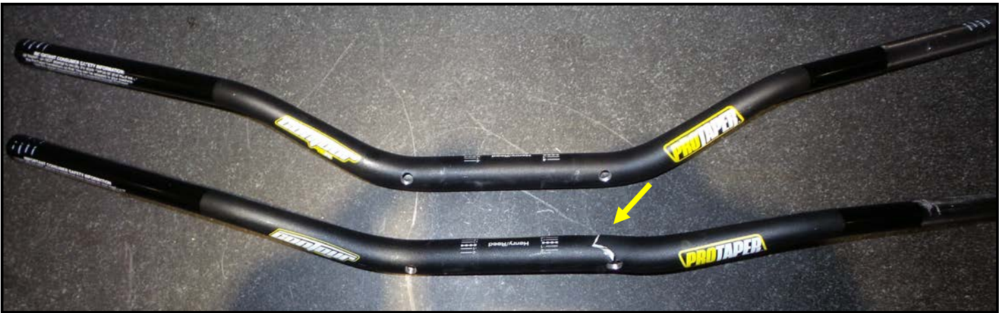
Figure 18 – Photo depicting Specialty sample post compression testing to failure, Top sample is not tested, Bottom sample depicting the permanent bending and fracture
