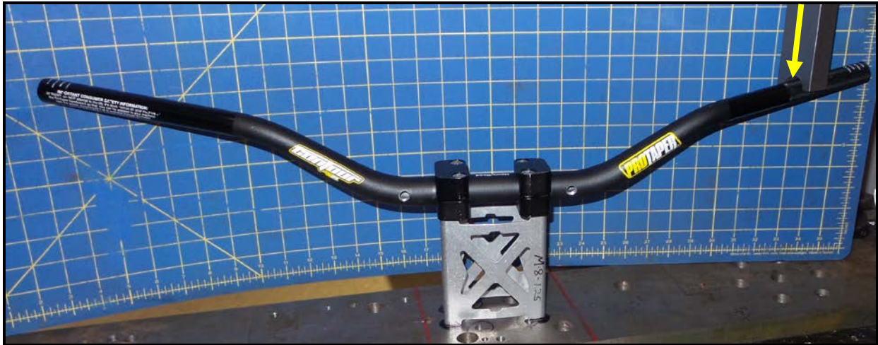
Figure 3 – Typical set up used for Method A, Top , Method B and Method C, Compression testing in direction of yellow arrow
