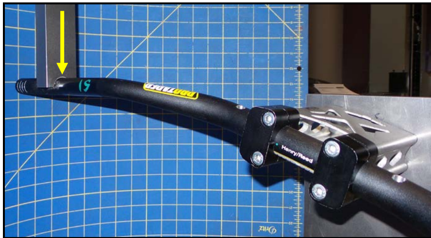
Figure 4 – Typical set up used for Method A, Front , compression testing in direction of yellow arrow
