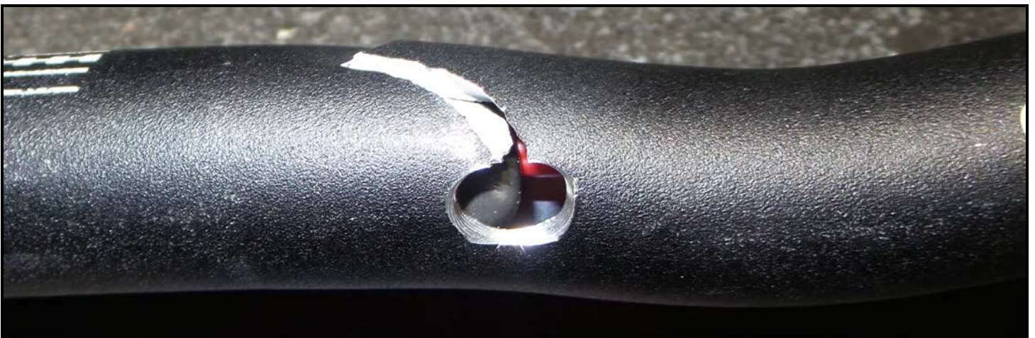
Figure 19 – Photo depicting failure mode magnified on the Specialty sample post compression testing to failure
