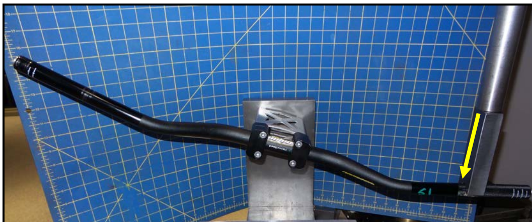
Figure 5 – Figure 6 – Typical set up used for Method A, Rear , compression testing in direction of yellow arrow
