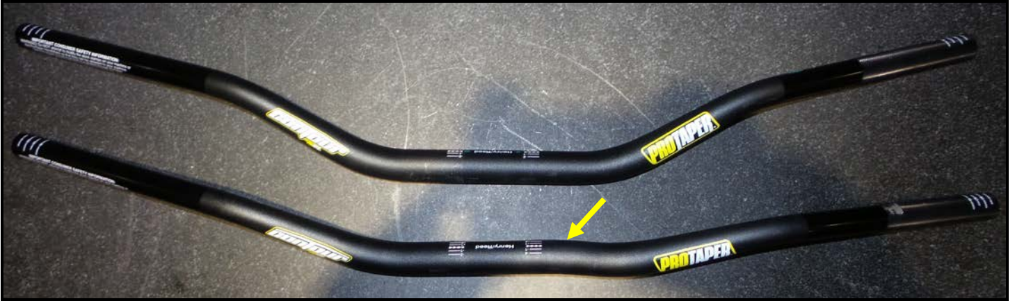
Figure 17 – Photo depicting Control sample post compression testing to failure, Top sample is not tested, Bottom sample depicting the permanent bending
